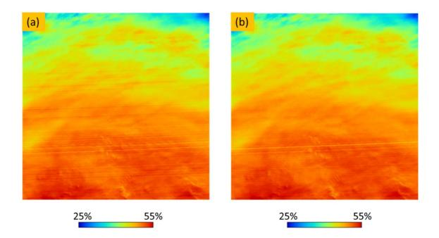
**Fig. 2.** (a) Albedos [%] of AHI-8 Band 2 at 03:10 UTC on 15 March 2016. (b) As per (a), but with bug-fixed calibration slope computation. The clear striping seen in (a) is mitigated in (b).
