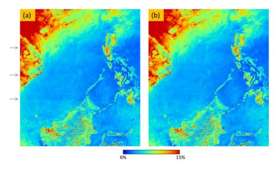
**Fig. 1** (a) Minimum albedos<sup>1</sup> [%] of AHI-8 Band 2 as extracted from 22 HSDs for 03:10 UTC from 10 to 31 March 2016. (b) As per (a), but with bug-fixed calibration slope computation. The extraction is performed at each HSD pixel for (a) and (b). The three clear lines observed at swath boundaries (i.e., banding) in (a) are significantly reduced in (b).
