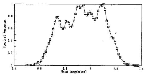
Fig.2.2.4 Spectral response of GMS-5 infrared channel 3
