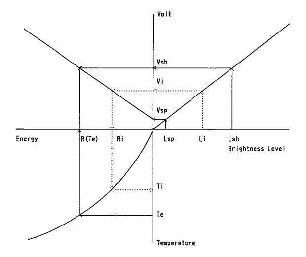
Fig.2.2.5 Infrared calibration procedure
