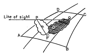
Fig.F.1 The illustration of the cloud projected on the earth surface. Q; apparent position of cloud.
