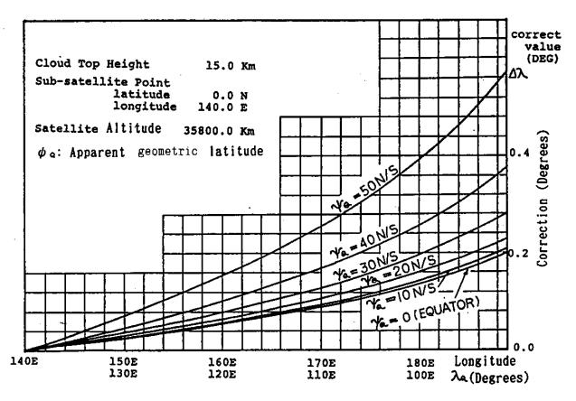
Fig.F.2 The correction curve for longitude-ways
