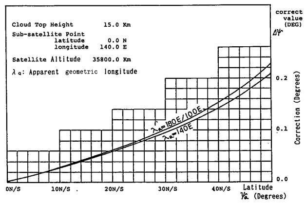
Fig.F.3 The correction curve for latitude-ways
