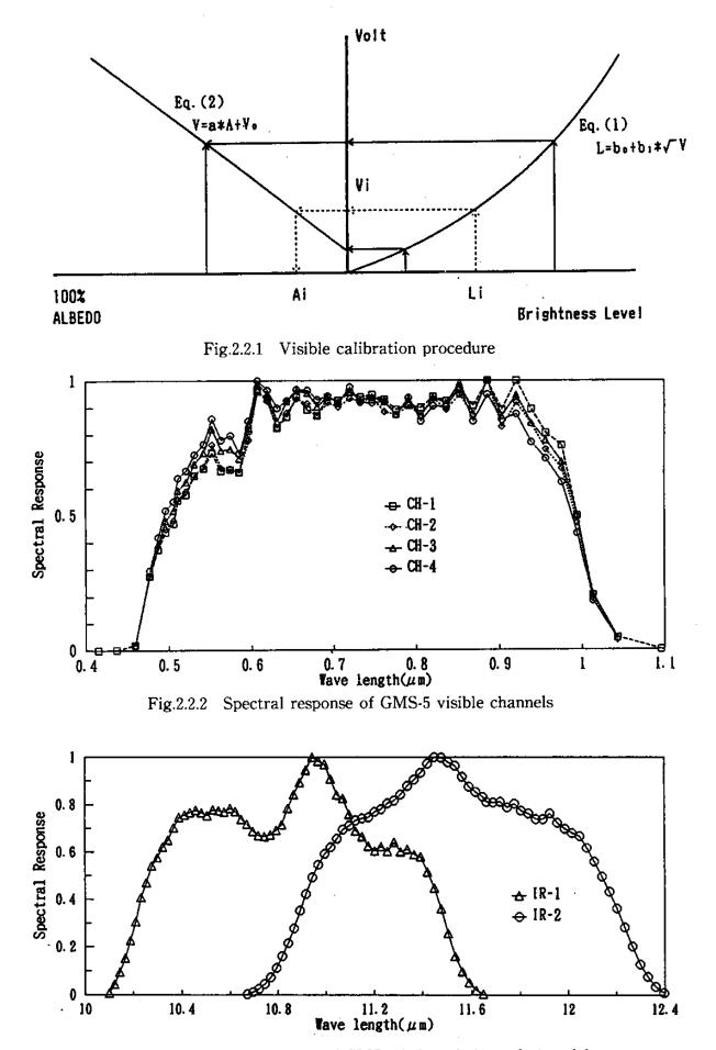
Fig.2.2.3 Spectral response of GMS-5 infrared channels 1 and 2
