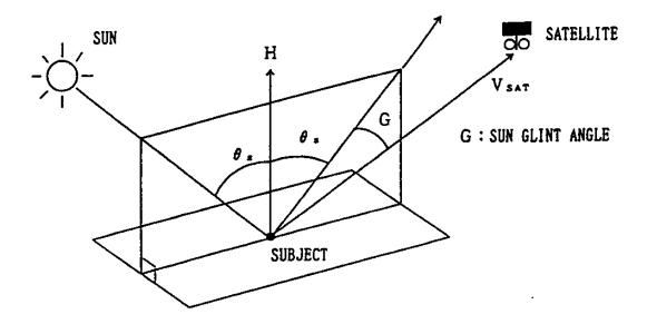
Fig.E.6 Sun glint angle, i.e., the angle between the vector of the sun's rays reflected at the subject and the vector from the subject to the satellite.
