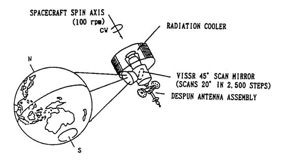
Fig.2.1.2 VISSR Spin-SCAN Geometry
