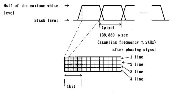
1 bit consists of 4 lines  $\times$ 4 pixel (4 lines repetition)
