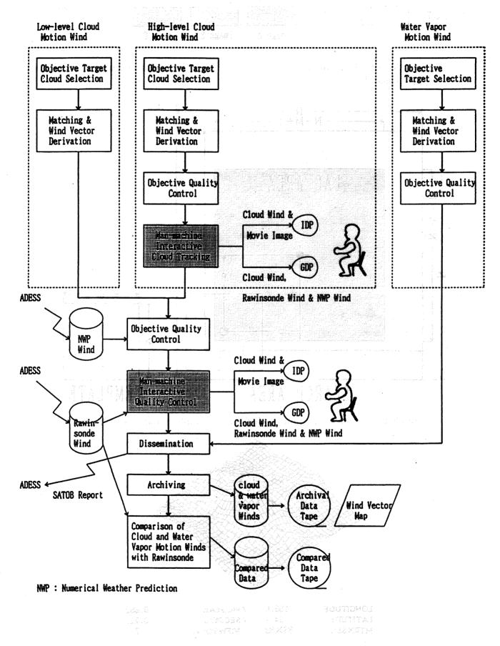
Fig.4.2.1 A flowchart of cloud and water vapor motion winds derivation system in MSC.
