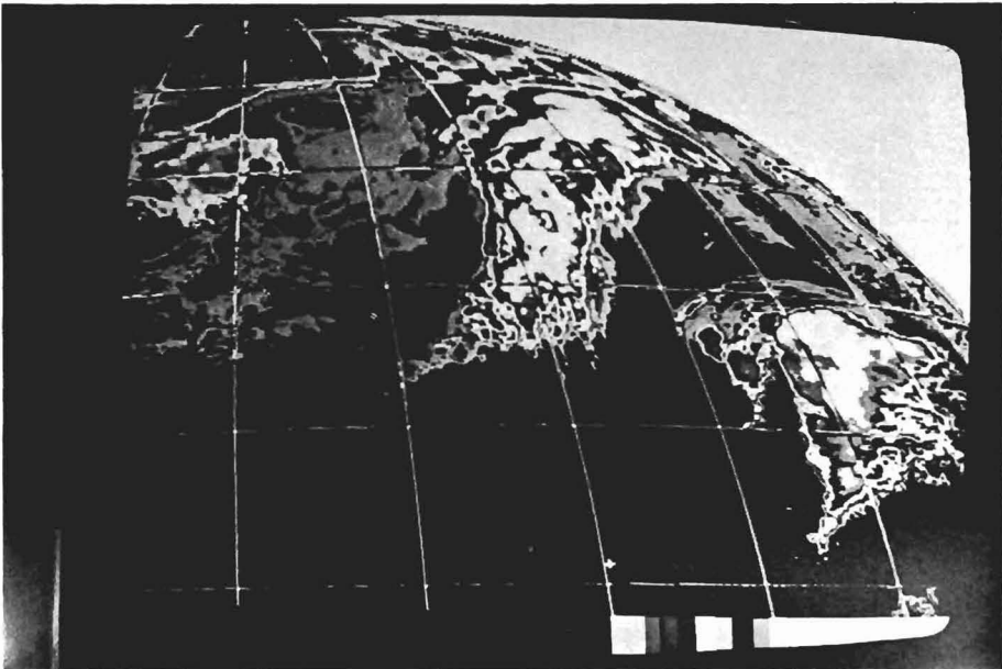
Fig. 26 Same as Fig. 12 except for enhanced image by false color system. As gray scale slicing is mainly applied to the cloud with lower temperature, Warm cloud in the southwestern part of cold front is obscure.
