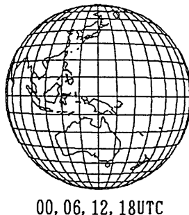
Figure-2 Illustration of diurnal change of view angle on the rectified earth image.
