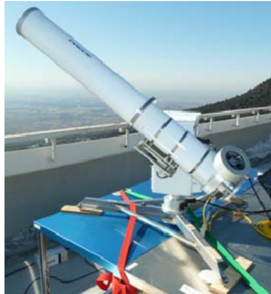
Photo 1 The collimation tube/pyranometer combination. A pyranometer with no sunscreen was attached to the bottom of the tube.
