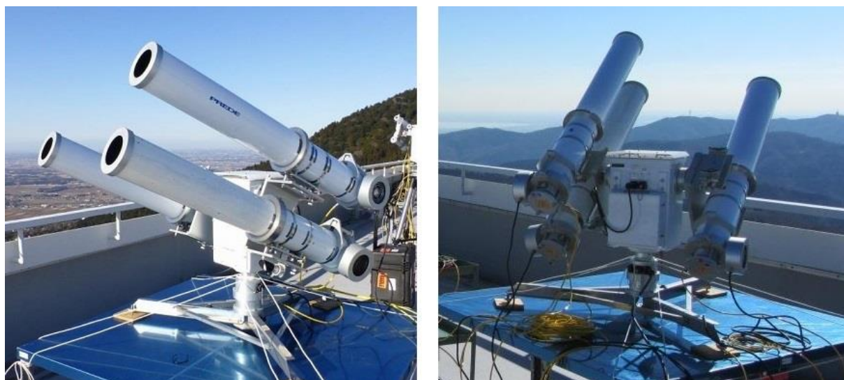
Photo 1 The collimation tube/pyranometer combination. A pyranometer was attached to the bottom end of the tube.
