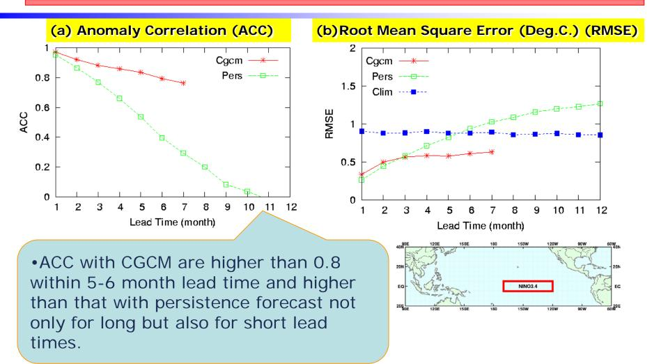
a) Anomaly correlation coefficients and b) RMSE of NINO3.4 index during 1984-2005 with respect to lead time after removing the mean bias. Red lines for JMA/MRI-CGCM, green lines for persistence forecast and a blue line for standard deviation of NINO3.4
