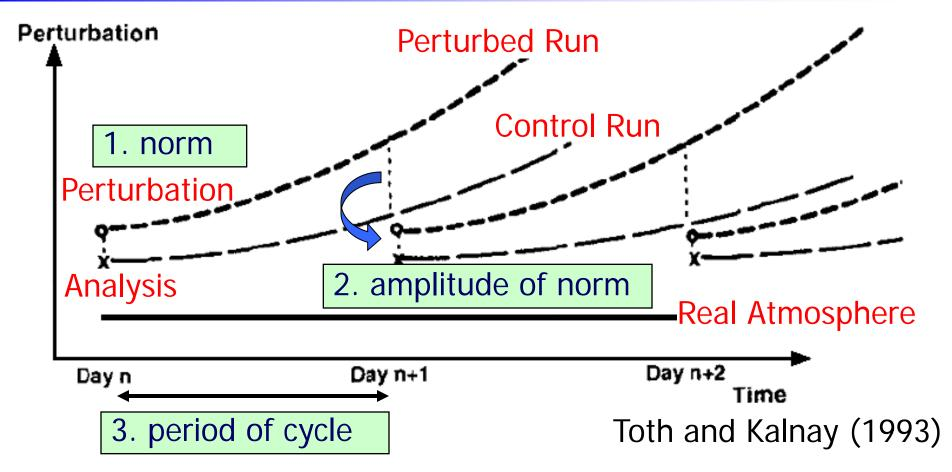
The model is integrated for 12 hours from the perturbed and the unperturbed initial conditions. The differences between the unperturbed control and the perturbed forecasts are normalized and used as an atmospheric perturbations.
