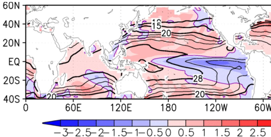
A systematic narrow bias in the simulated meridional width of the SST anomalies of ENSO has been seen in JMA/MRI-CPS2 and most of CMIP5 models. (Zhang and Jin 2012) Corresponding to the SST pattern, active convection are predicted over latitudinal band of about 5 – 15N in the North Pacific.
