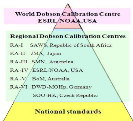
Figure 9 Calibration system of Dobson spectrophotometers
